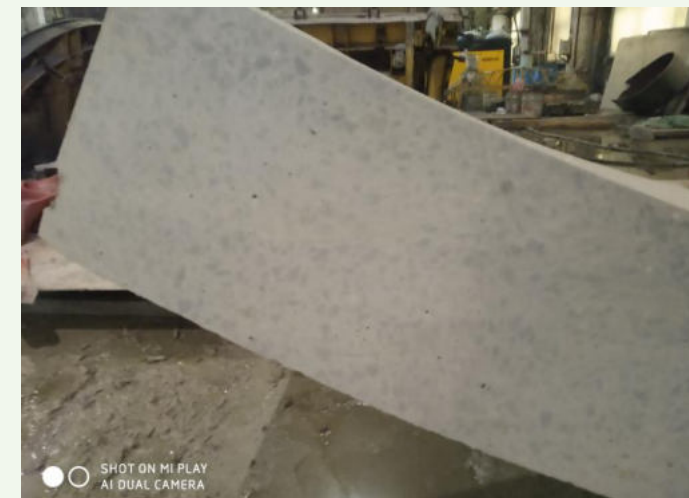
Cross-section of concrete segment Good quality of pouring
