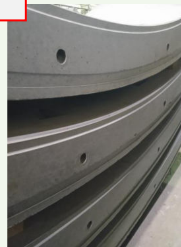
Segments after demolding Good surface
