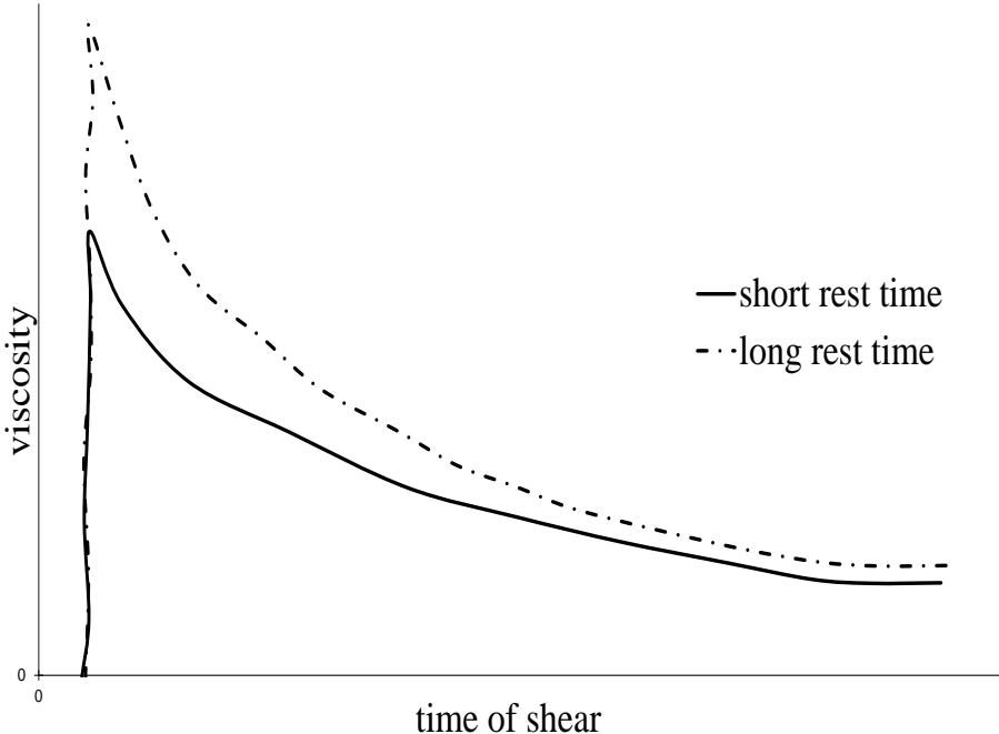
Viscosity as a function of shearing and resting time before shear
